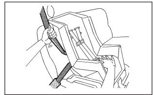
6. To tighten the belt, push down on the child restraint, pull the shoulder belt to tighten the lap belt portion and feed the shoulder belt back into the retractor. If you are using a forward-facing child restraint, you may find it helpful to use your knee to push down on the child restraint as you tighten the belt. You should not be able to pull more of the belt out of the retractor once the lock has been set.
